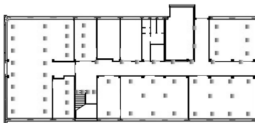
Fig. 2. Layout of the WSN testbed.
